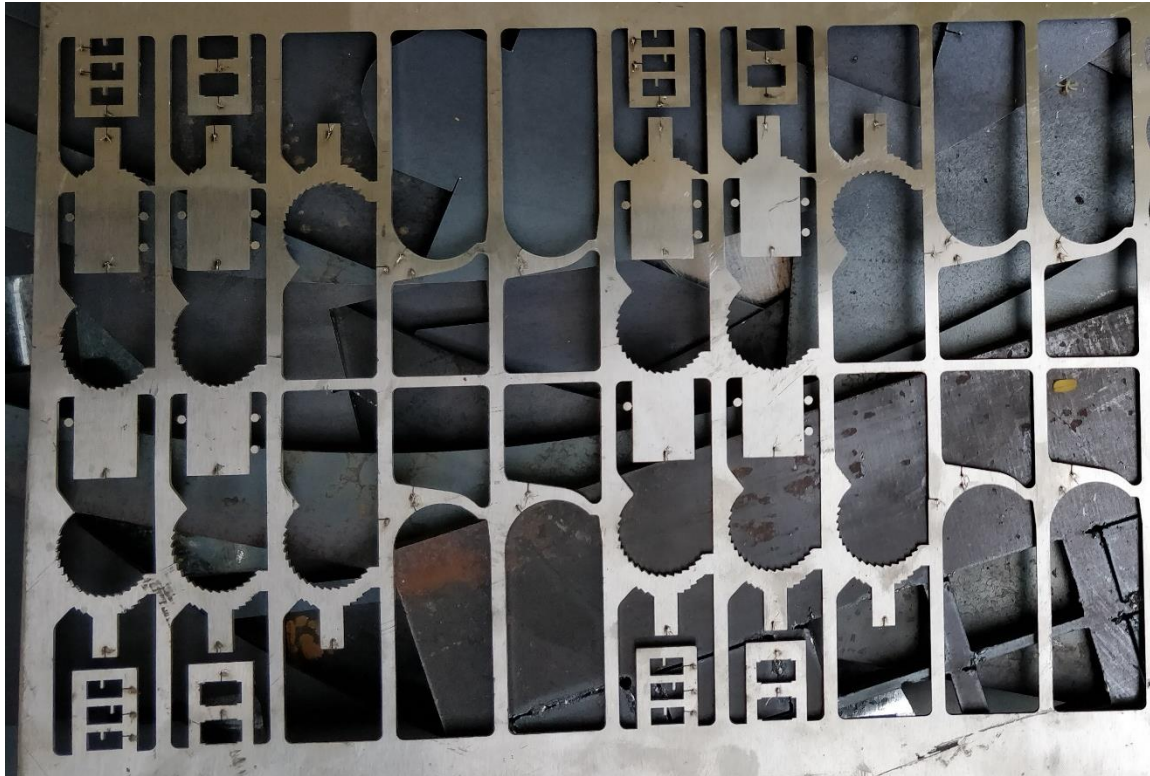
Figure 3.16: Cut-out on sheet after laser cutting
